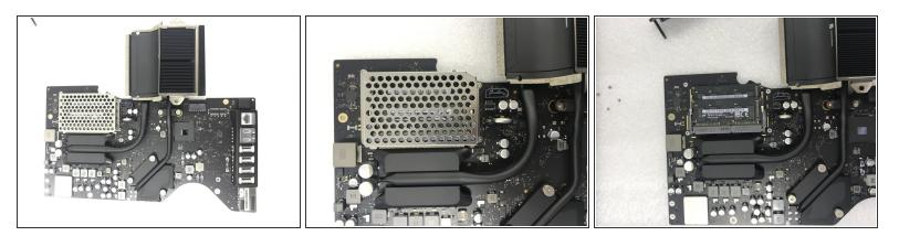
• A protection cover for the RAMs which I think is not necessary for a fixed device like this and as you know 2666 MHz DDR4 rams are little higher speed than the 2017 model.
