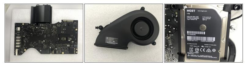
• Only wifi and bluetooth module in now fixed on the board. Hard drive still same Hitachi 5400 rpm and fan still the same as you can see
