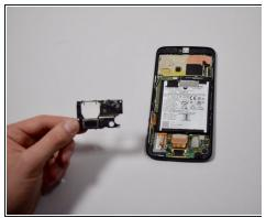
• Use the nylon spudger to lift and remove the speaker from the phone chassis.
