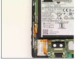
Using the spudger, lift up the bar on the ZIF connector that joins the ribbon cable to the control buttons.
