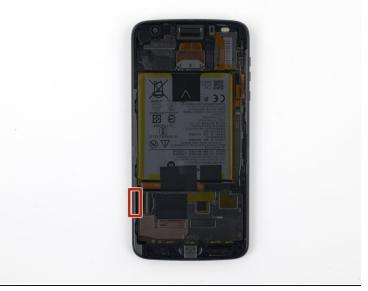
When separating the left side of the screen assembly, take care to not snag the display cable located on the left edge near the bottom of the display.
