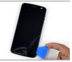
Slide your opening pick all along the right side of the device to release the clips and adhesive securing the screen assembly.
