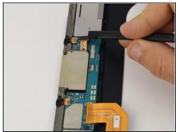
• Disconnect the single press fit connector located just above the Micro SD card tray on the left midframe.
