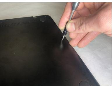
Remove all ten 5mm screws from the backplate using a Phillips #0 Screwdriver.
