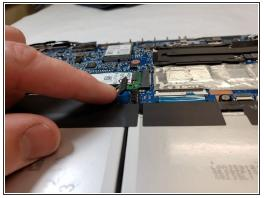
• Disconnect the battery from the laptop in the upper left side of the battery, using tweezers.
