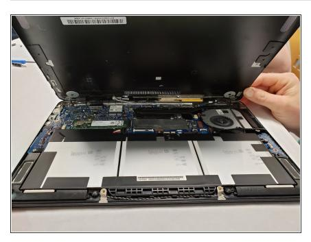
Lift up the back plate and slide it to the back of the computer to remove.
