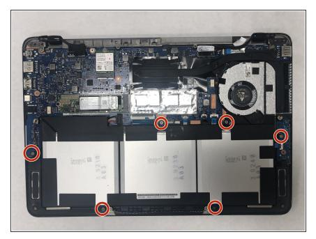
Remove the six 5 mm screws holding the battery using a Phillips #0 screwdriver.
