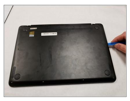
Carefully remove the backplate using the plastic opening tool.
