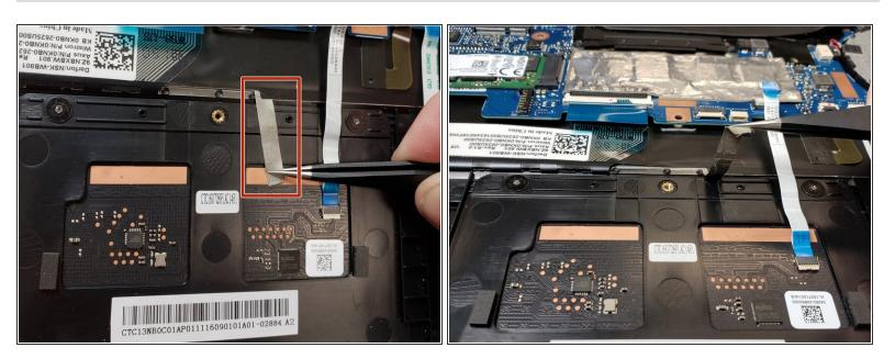
Remove adhesive tape tethering the trackpad to the motherboard with tweezers.
