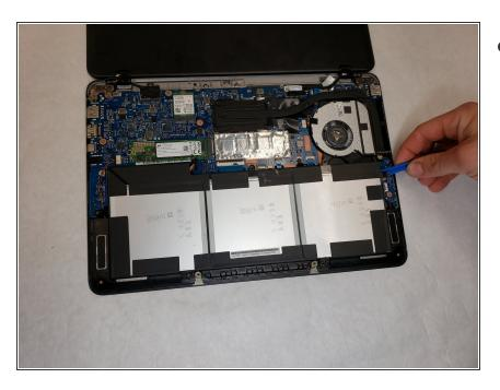
Carefully remove the battery using the plastic opening tool.
