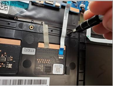
Remove the two 5mm screws holding in the trackpad using a Phillips #0 screwdriver.
