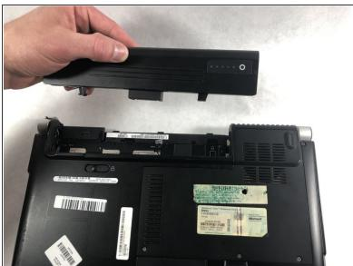
• Lift the computer up and slowly pull the battery straight out from the device.
