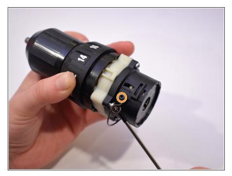
Use a screwdriver to pop the speed selector lever off to gain access to the screws underneath it.
