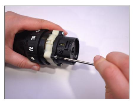
Use a screwdriver to remove each of the four 6mm screws holding the gear case assembly in place.
