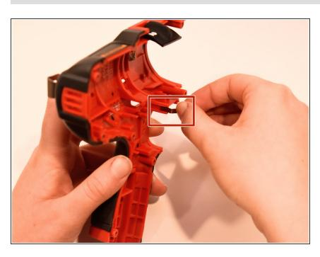
Remove the spring plate and insert replacement spring plate.
