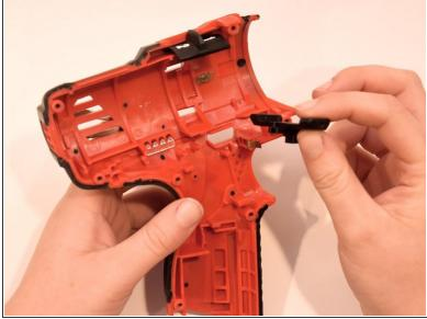
Remove the forward/reversing shuttle to gain access to the spring plate.
