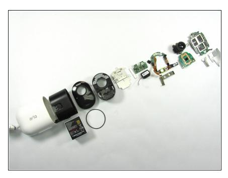
Teardown Exploded View of the Arlo Ultra 4K Wire-Free HDR Security Camera
