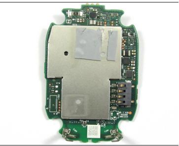
• The Main PCB has EMI / Heatsink Shielding on the frontside and backside
