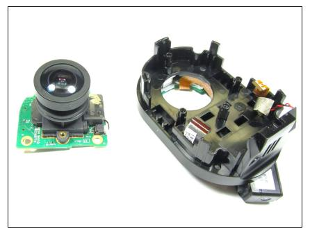
After the Flex PCB has been removed, the Camera Lens plus Image Sensor PCB can be gently pulled out from the Camera Assembly Body
