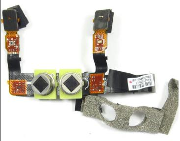
• After removing the the Flex PCB, remove the Metal Shield Tape from the Flex PCB
