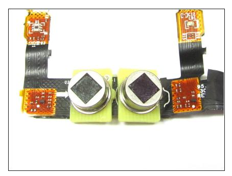
PIR Sensors, Light Detector, and Mutli-Color LED Close up View
