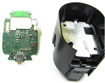
• Remove the Main PCB from the Camera Body by gently prying it out using the Spudger Tool
