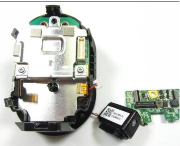
• With the Spudger Tool, pry out the Small PCB on the back of the Camera Assembly
