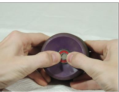
Wedge each bearing back into the center of the wheel.
