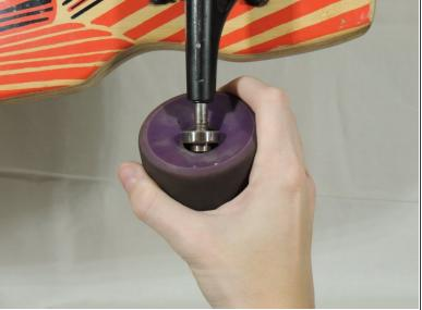
• Use the axle to carefully pry each of the bearings out of the inside of the wheel.
