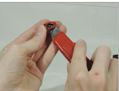
Remove the rubber seal fitted in the bearings with a thin blade.
