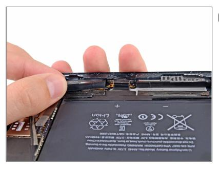
During reassembly, make sure the two speaker contacts are placed above and below the screw hole on the Lightning connector.
