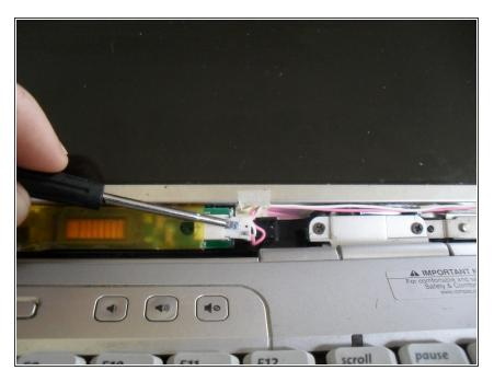
Remove the backlight inverter cable using a spudger or flat blade screwdriver
