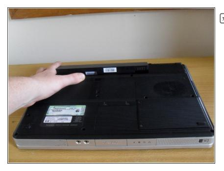
Remove the battery before starting working on the laptop
