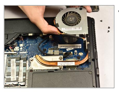
• Gently lift the fan straight up until it is lifted out of the case.
