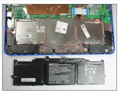
• Remove Battery Assembly from device.
