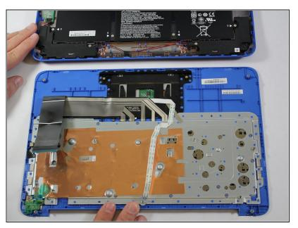
• Remove the Keyboard/Top Cover from the device.
