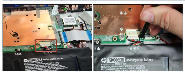
Use a pick to detach the Battery assembly cable.
