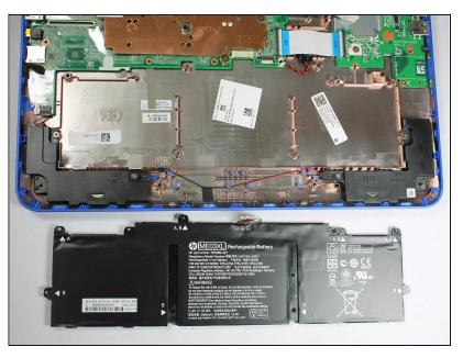
• Remove Battery Assembly from device.
