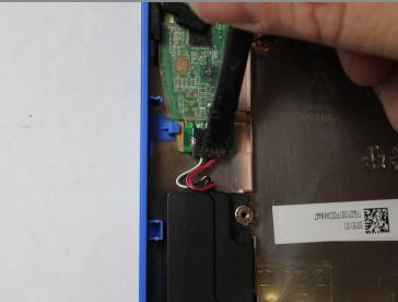
Use a pick to disconnect the Speaker Cable from the System Board.
