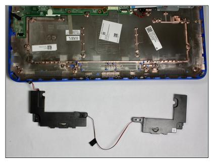
• Remove the Speakers from the device.
