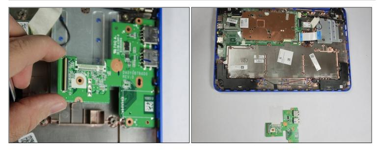
• Remove the USB/Card Reader board assembly from the device.
