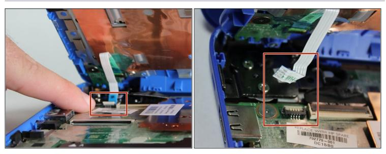
• Disconnect the Power connector cable.
