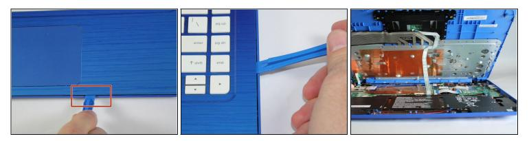
• Insert the Spudger between the Top Cover and Bottom Cover to lift the front edge until it separates from the Bottom Cover.
