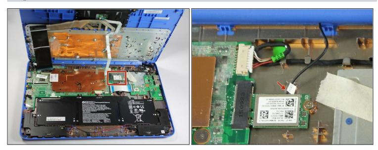
• Disconnect the WLAN antenna cable from the WLAN module.
