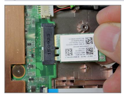
• Remove the WLAN Module from device.
