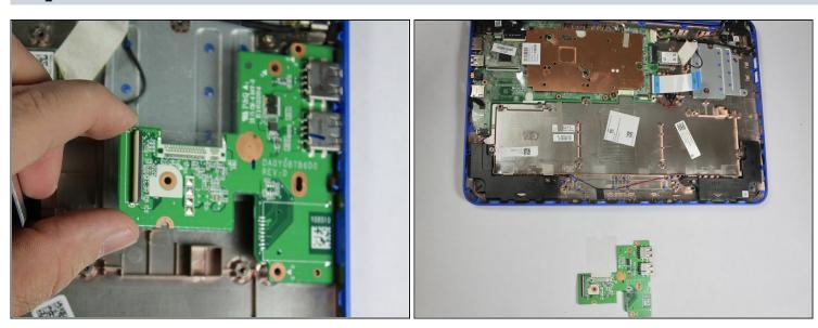
• Remove the USB/Card Reader board assembly from the device.
