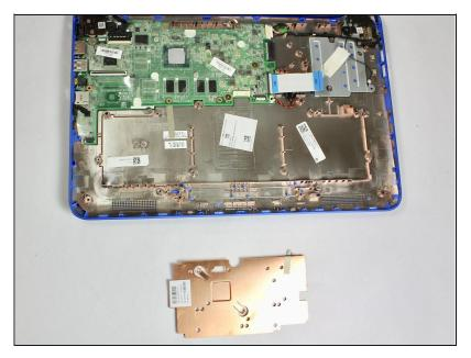
Remove the Heat Sink from the System Board.
