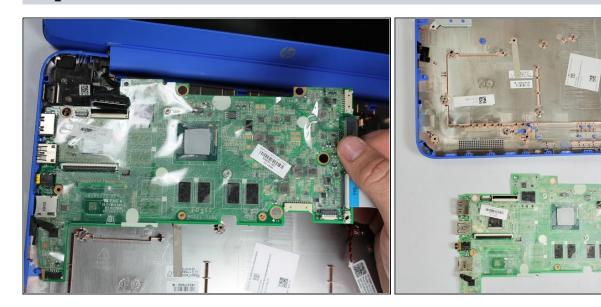
• Lift the right side of the System Board and slide it from the device.
