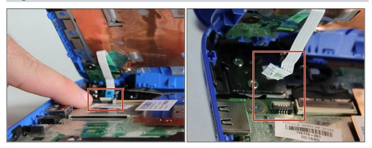
Disconnect the Power connector cable.
