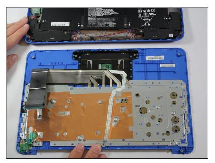
• Remove the Keyboard/Top Cover from the device.
