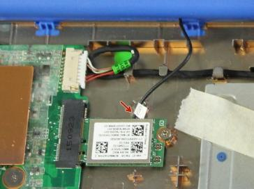
• Disconnect the WLAN antenna cable from the WLAN module.
