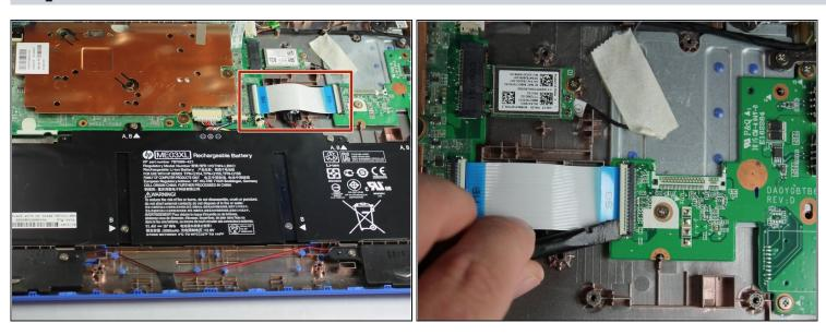
Use a pick to disconnect the USB/Card Reader cable from the System Board.
