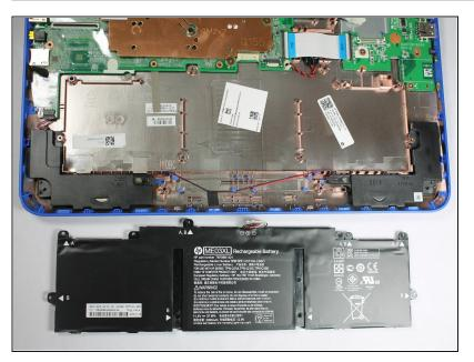
Remove Battery Assembly from device.
