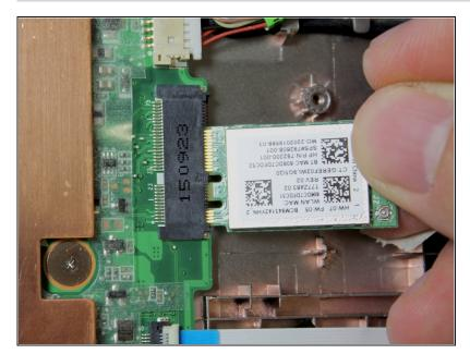
• Remove the WLAN Module from device.
