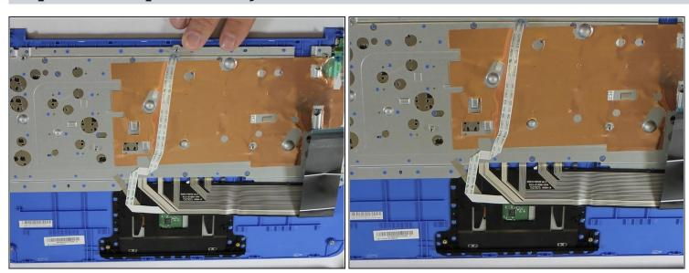
• Place the Top Cover/Keyboard assembly face down with the front towards you.
