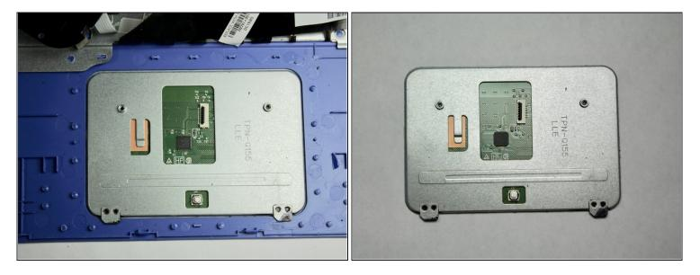
Remove the Touchpad assembly from the device.
