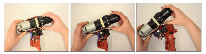
• Remove the unit from the housing assembly and set the housing assembly aside.
