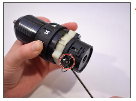
Use a spudger to pry the broken speed selector lever off the assembly.
