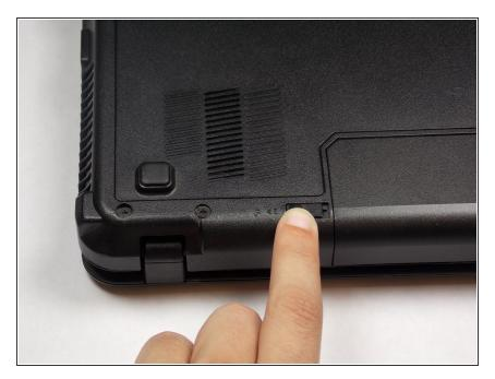
Push and hold the switch on the left to its "unlock" position.
