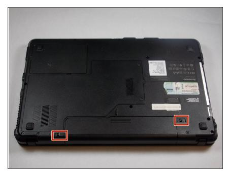
Locate the switches on the bottom of the computer on either side of the battery, as shown in the picture.
