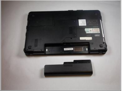
• While still holding the switch on the left in the unlock position, slide the battery out.
