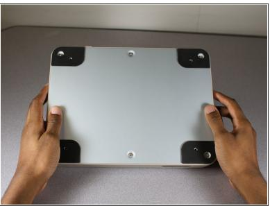
Turn the device over so that the bottom of the device is facing up.
