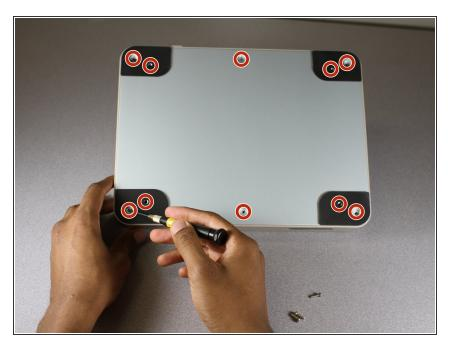
Use a Phillips #0 screwdriver to remove all ten of the 3 mm screws on the back plate.
