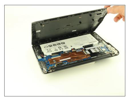
Lift the case up and off the device
