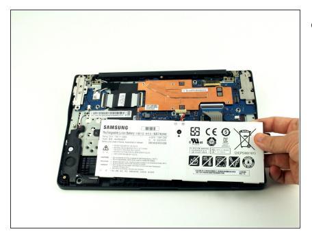
Lift the battery up and out from the case.
