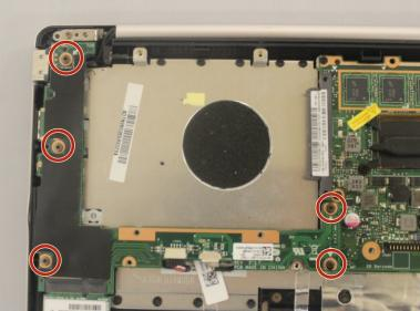
Unscrew the five 5mm screws holding the left board together.
