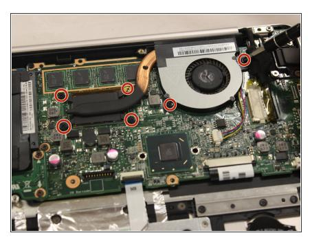
Remove the six 4mm screws holding the fan and CPU cover.
