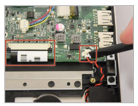
Remove the two remaining connectors on the board.
