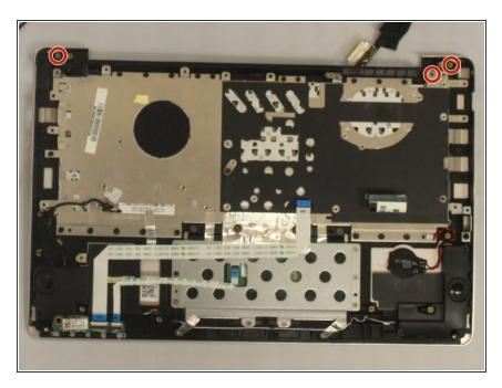
Unscrew the three 5mm screws holding the display to the main body of the computer.
