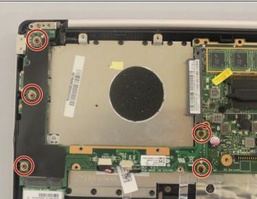
Unscrew the five 5mm screws holding the left board together.
