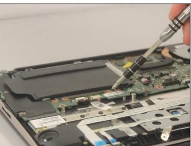
Unscrew the three 4mm screws holding the hard drive to the board.
