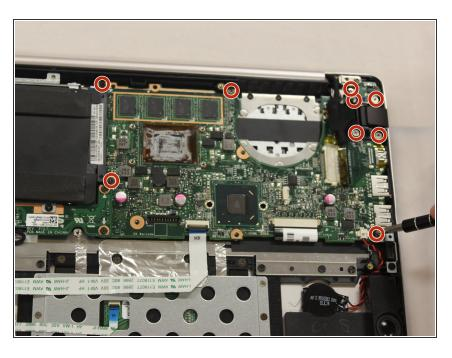
Unscrew the nine 4mm screws holding the right board together.
