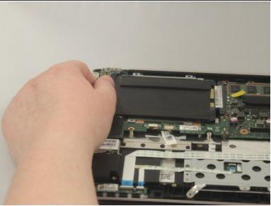
• Pull on the tab on the left side of the hard drive and slowly disconnect it from the board.
