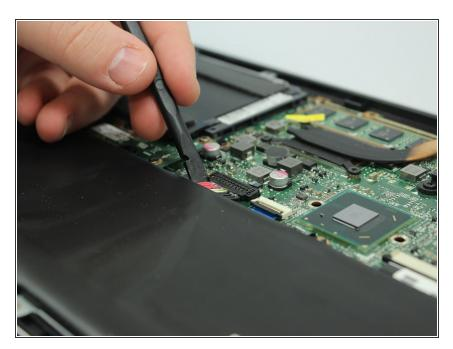
Disconnect the battery ribbon cable from the motherboard.
