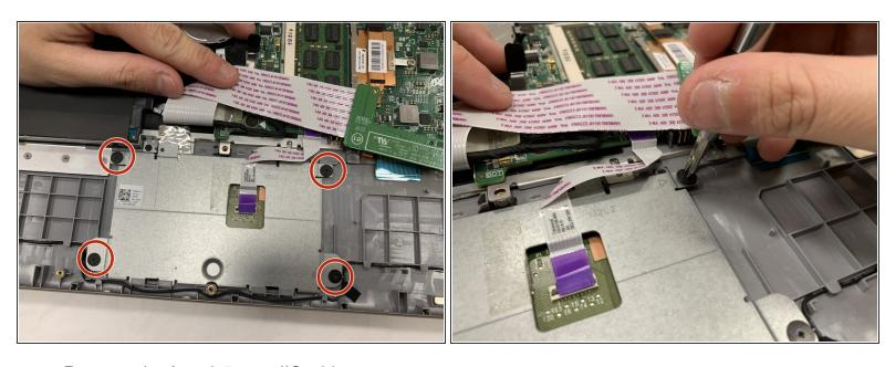
Remove the four 2.5 mm JIS #00 screws.
