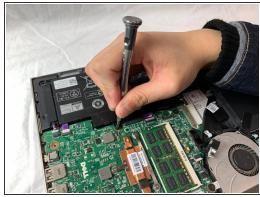
Remove the three 4 mm JIS #00 screws that secure the battery to the device.
