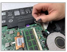
• Unplug the flat connector that is connected to the battery.
