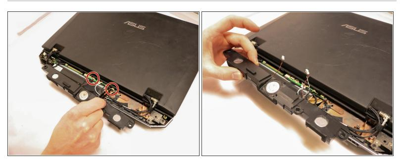
Using the bent black tweezers, remove both wires connecting the sound bar to the motherboard.
