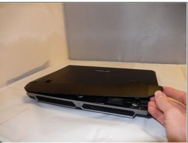
Using the iFixit opening tool, gently pry open the plate covering the spine of the device.
