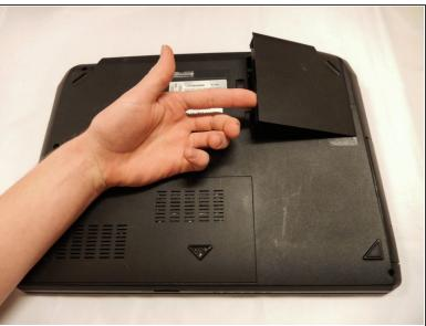
Side the switch and lift the battery from the back of the device.
