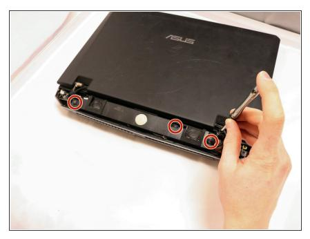
Using the PH 00 screwdriver, remove the three 10.6 mm screws holding the sound bar down.
