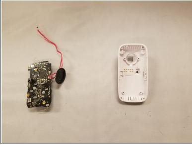
You will now be able to carefully pull the receiver wire through the gap in the casing.
