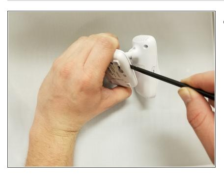
Use a nylon spudger to remove the casing.
