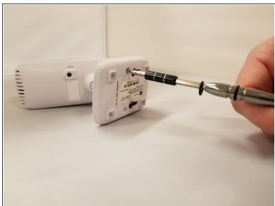
Remove two 5 mm Phillips #1 screws from the bottom of the camera stand.
