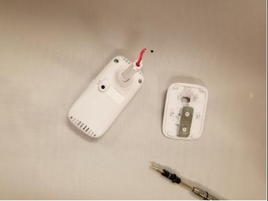
Now, remove the bottom of the stand by pulling it from the camera.
