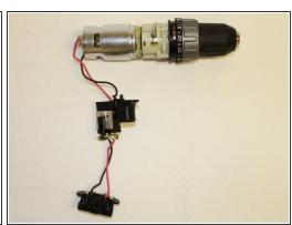
Remove the switch assembly, chuck, and motor from all drill covers.
