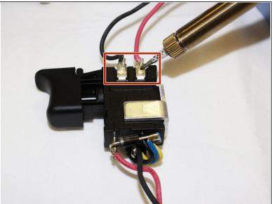
To replace the switch assembly, desolder the black and red wires and replace with a new switch assembly.
