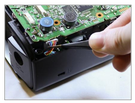
• Disconnect the bundled cables leading to the printing mechanism.
