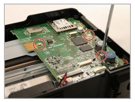
• Unscrew the three 3mm PH000 screws from the motherboard.
