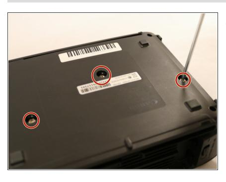
Unscrew the three 4mm PH1 screws on the bottom of the printer.
