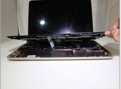
After ribbon cables have been disconnected, carefully lift up keyboard to disconnect from base of laptop. To reassemble your device, follow these instructions in reverse order.
