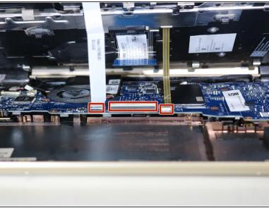
Disconnect the three connected cable ribbons connected to the motherboard by gently pulling them out of their connectors.
