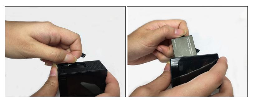
• Locate the small plastic flap attached to the battery. Pull the battery out towards you.
