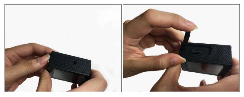
Locate the battery cover at the bottom of the camera. Use your fingers to gently pry open the battery cover.
