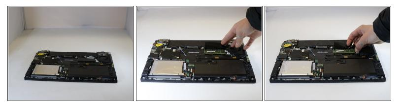
• Pull one side of the prong that is holding the RAM in place
