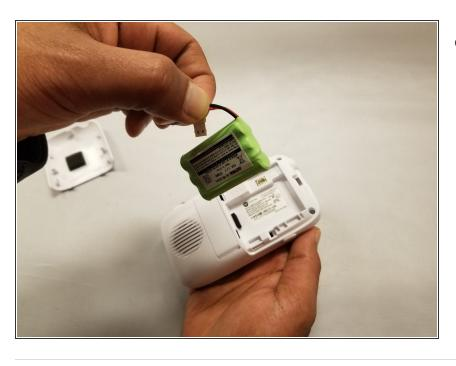
Remove and discard the old battery and replace it with a new battery.
