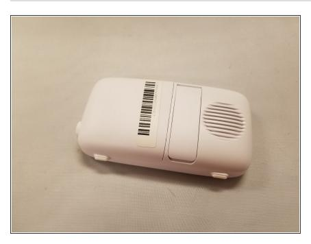
The battery casing is on the back of the monitor housing.
