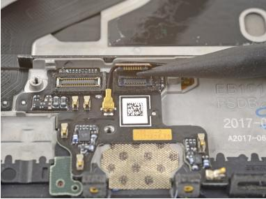
Use the point of a spudger the pry up and disconnect the fingerprint scanner connector from its socket on the daughterboard.
