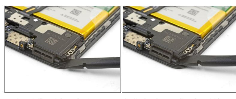
Insert the flat end of a spudger into the corner of the loudspeaker assembly and pry slightly, loosening the loudspeaker from its recess.
