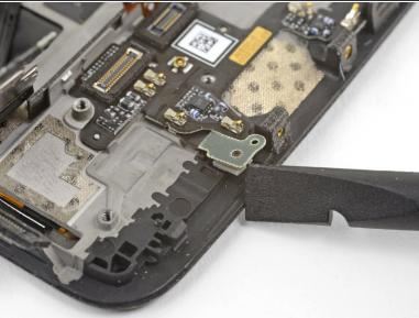
• Insert the edge of a flat end of the spudger underneath the microphone board and twist slightly to release the board's adhesive.
