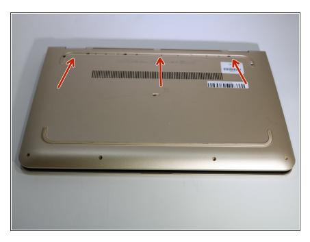
Remove rubber foot closest to computer hinge with a Metal Spudger.
