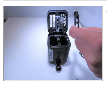
Remove the two screws down the middle and lift the middle component off
