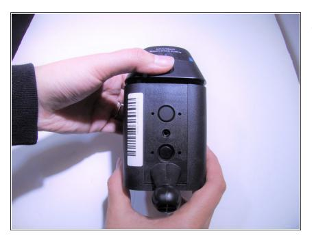
Press down on top button and open upward
