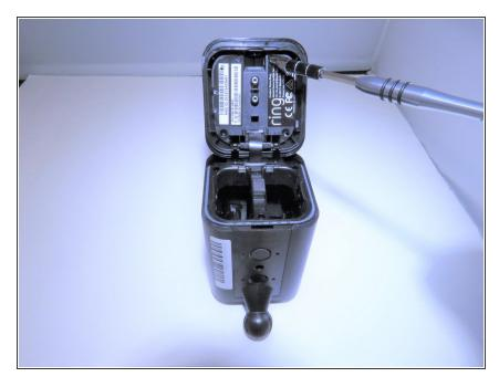
Remove the remaining 10 screws that are around the border under the tape.
