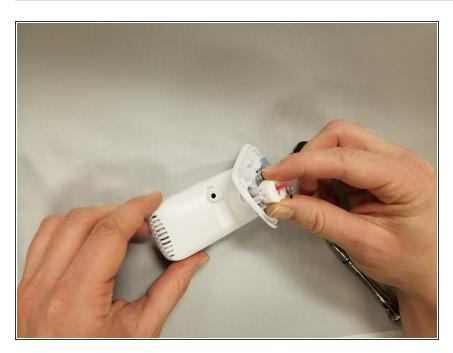
Remove the white plastic wire housing beneath the black plastic.
