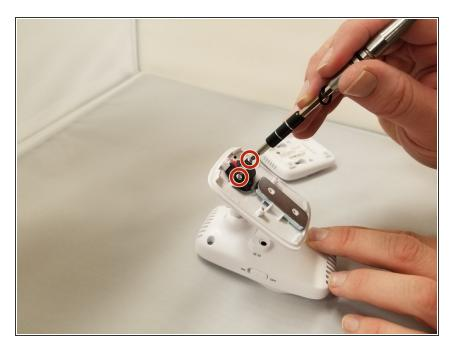
Remove the two 5 mm Phillips #1 screws attached to the black plastic under the casing.
