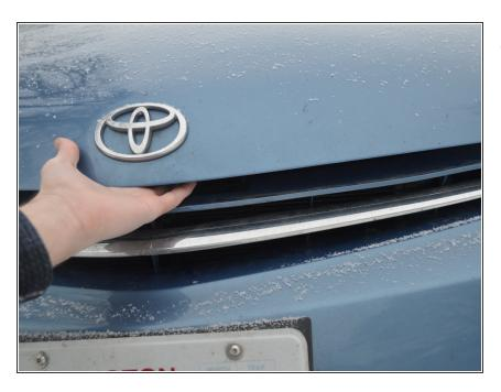
Reach under the hood and find the lever that releases the hood. push up on it and lift the hood.
