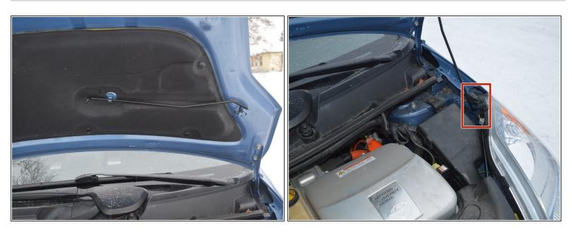
Unlatch the metal rod and place it in the designed area so it will hold up the hood.
