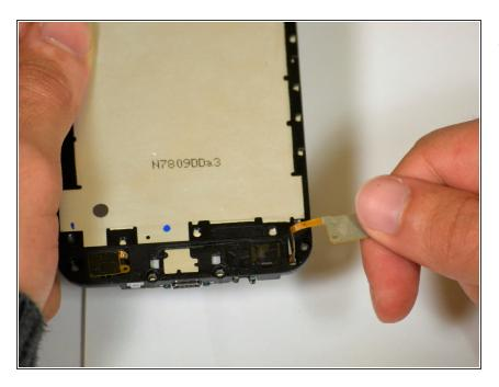
Lift up the connector and push it through the motherboard by following the ribbon.
