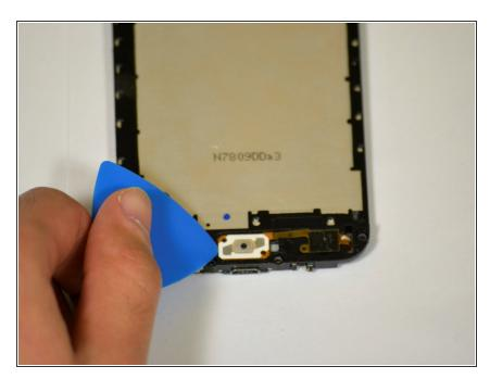
Remove the connector where the home button was using the iFixit Opening Pick.
