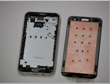
Pry the connector off of the motherboard by using a clean nail or the iFixit opening tool.
