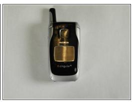
Snap the top cover into place so that the outside screen is visible. Press around the perimeter to secure the case.
