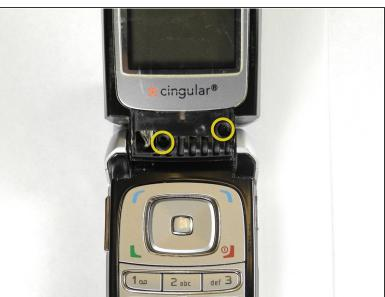
Open the phone and insert the screws tightly.
