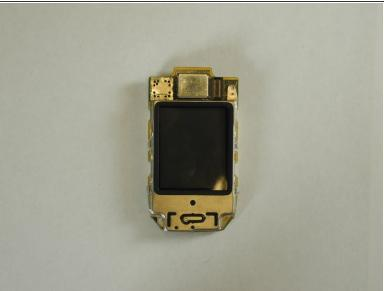
Place the metal case over the top of the screen so that it snaps into place.
