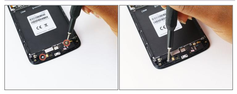
Remove the two 4mm silver screws holding down the charging port board with Phillips bit.
