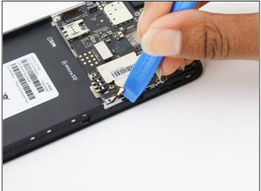
• Disconnect the <u>antenna cable</u> by sliding a plastic pry tool or fine tweezers under the wire close to its socket, and then prying straight up.
