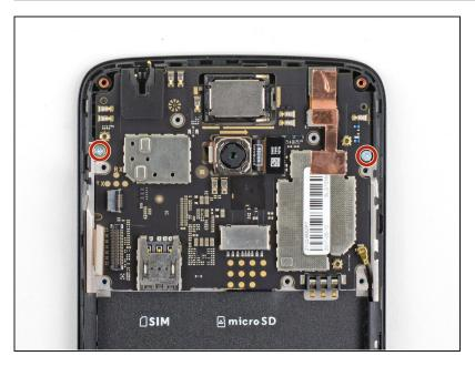
Remove the two 3.1 mm long Phillips screws securing the motherboard.
