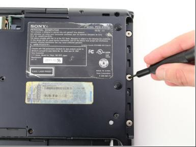
Remove the three 2mm Phillips #00 screws located on the top right edge.
