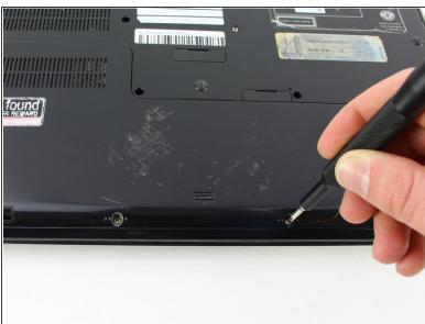
Remove the two 3mm Phillips #0 screws on the bottom of the computer that secure the plastic backing.
