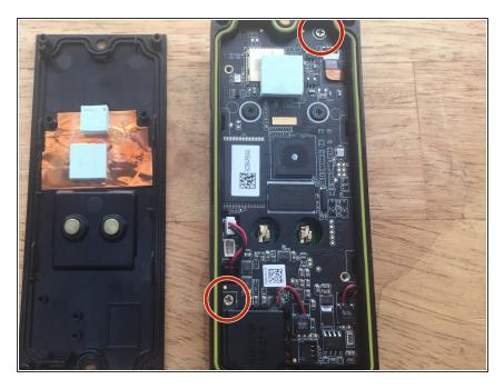
Remove the two silver Phillips screws holding the motherboard in place.
