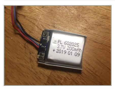
After the necessary soldering has been done, carefully fold the battery circuit to where it is tucked into the battery.
