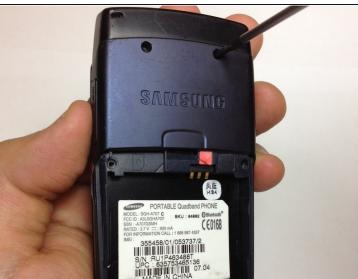
Unscrew the six screws on the back of the phone using the Phillips #0 screw driver.
